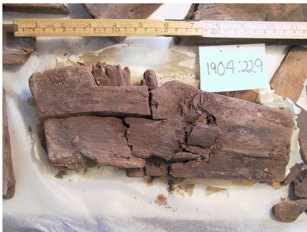
Figure 1 A piece of alum-treated wood from the Oseberg find. The cracks show how fragile most of the wood is. Note that the acidity of the piece has even caused the original paper that the piece was stored on to degrade (© Museum for Cultural History, University of Oslo).
